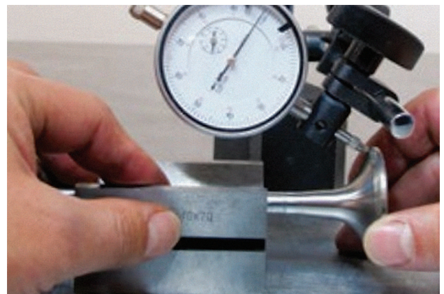
Figure 3: Measuring valve seat surface runout.
