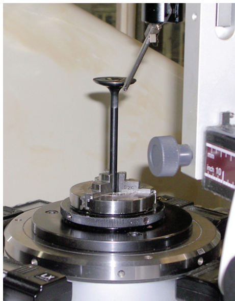
Figure 4: Valve seat roundness measuring equipment
