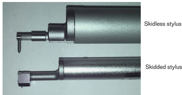
Figure 12. Two types of stylus instruments. The skidded type is most common for production cylinder bore measurements. Courtesy The Surface Texture Answer Book*.
