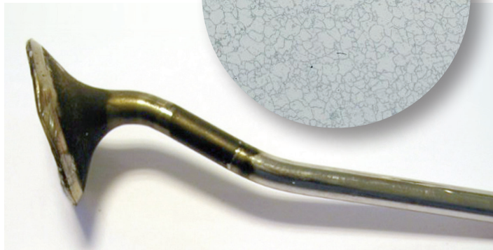
Figure 2. Microstructure of 21-4N steel with low carbide precipitation and ductile response after an impact with the piston.
