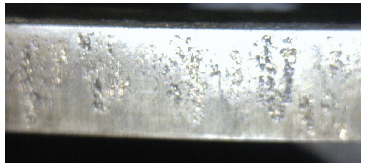
The faces on the top and intermediate ring have been destroyed.
