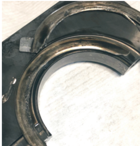
Failed Thrust Bearing
