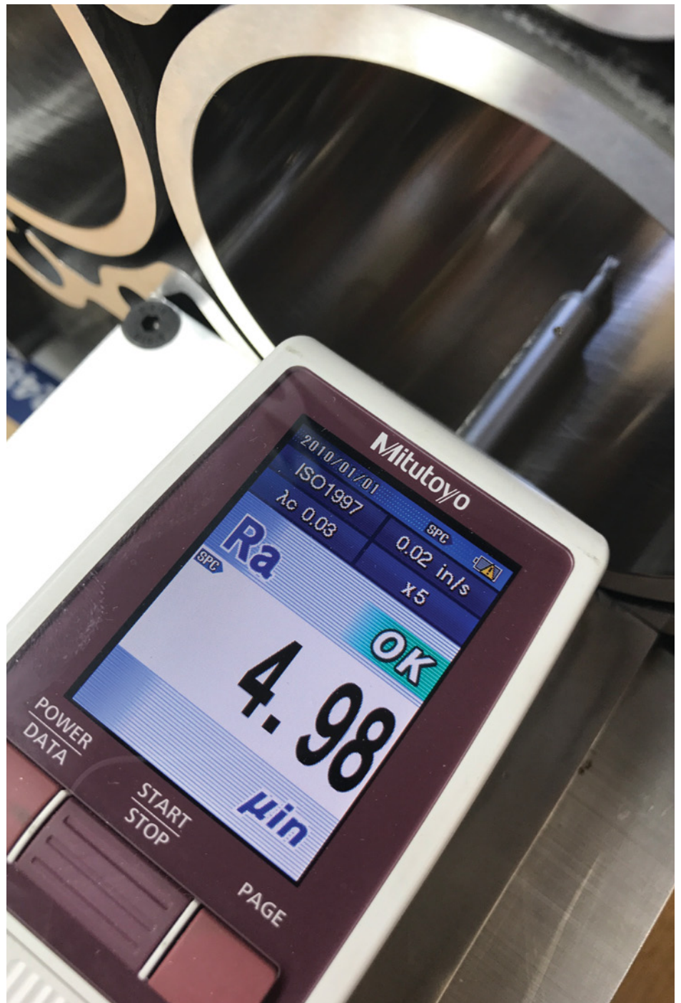
Figure 4. SJ-210 Profilometer Nikasil Surface Trace
