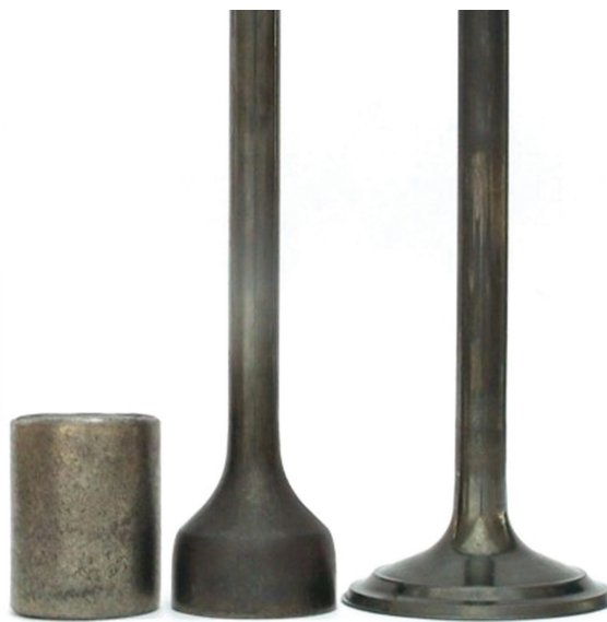
Figure 1: From left to right, cut bar, extruded product, and forged valve
