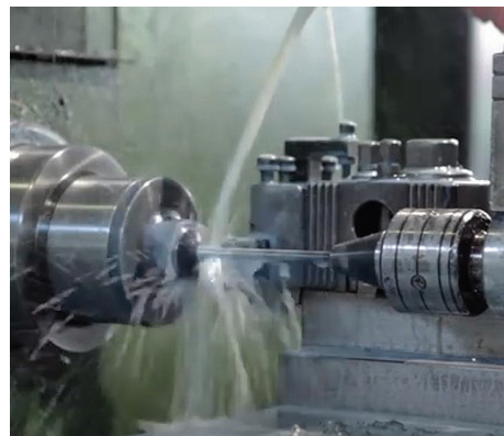
Figure 21: Fillet radius CNC turning
