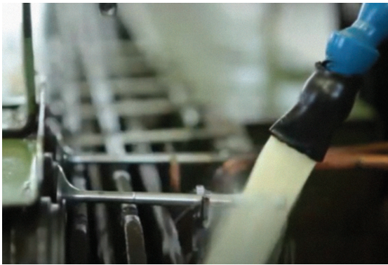
Figure 25: Tip and grooves quenching
