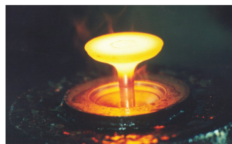
Figure 9: Forged valve extracted from the press
