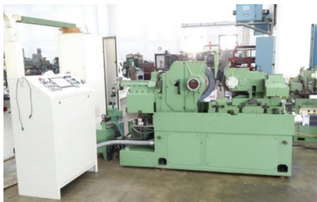
Figure 18: Typical centerless grinder, with the grinding wheel at the middle left.
