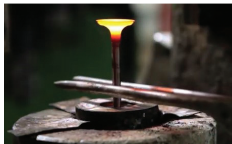
Figure 8: Finished forged valve
