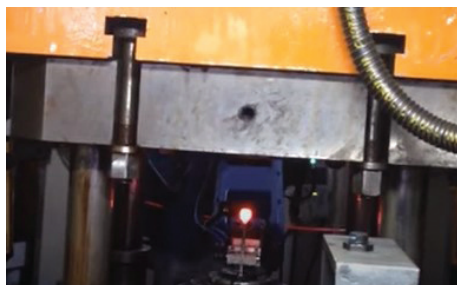
Figure 7: Valve just before being stamped in the press
