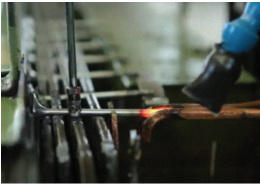
Figure 24: Tip and grooves induction heating
