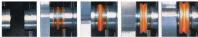
ABOVE: Figure 15: Friction welding steps (Left side rotates and pushes against fixed right side). BELOW: Figure 16: Construction steel bar "pin" welded to a highly alloyed steel "head".
