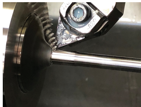
Figure 22: Taper stem end and fillet radius CNC turning
