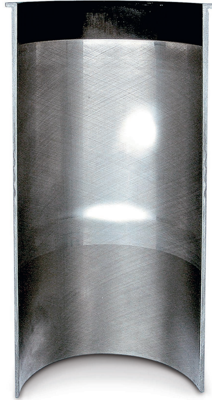
Wear on the sliding surface due to distortion
