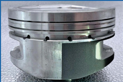
"Detroit Street Outlaw" Jr. Southwell's scuffed, worn pistons 225 passes ProCharged SBF restored by adding .012"+ coating Appearing on Discovery Channel's "Fastest in America" Fall 2021
