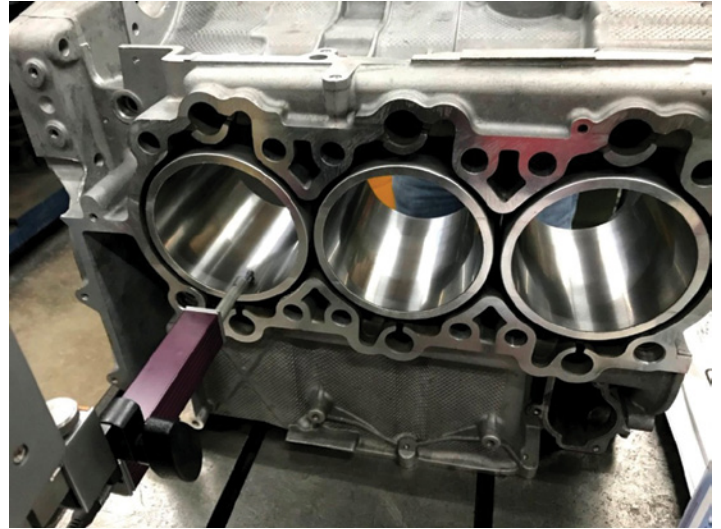
Porsche M96 block with aluminum wet sleeve with SUMEbores APS coating.
