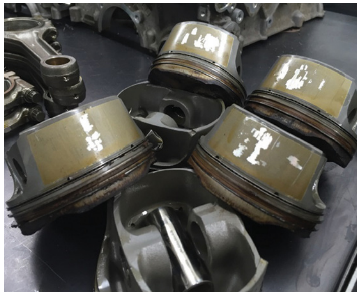
Failed piston skirt coating.
